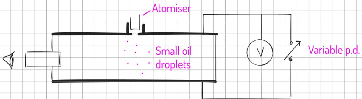
Electric field off. Droplet falls freely and reaches terminal velocity.
