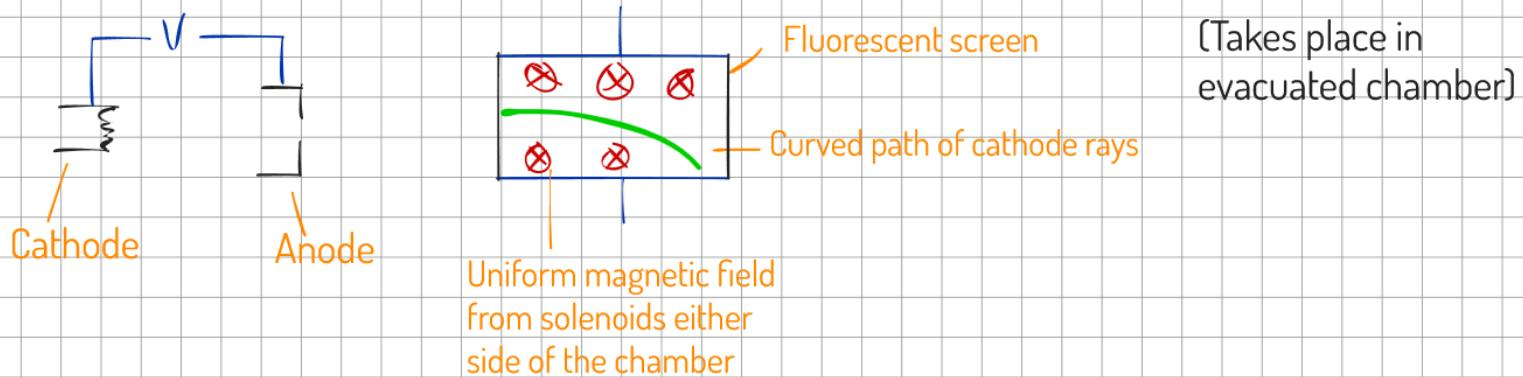
Force from the magnetic field causes the cathode rays to follow a circular path.
