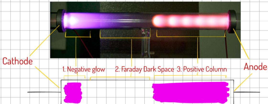
3. Excitation of electrons in the gas atoms due to collision with electrons that have been accelerated from the cathode. Glow is due to photon emission during deexcitation.
